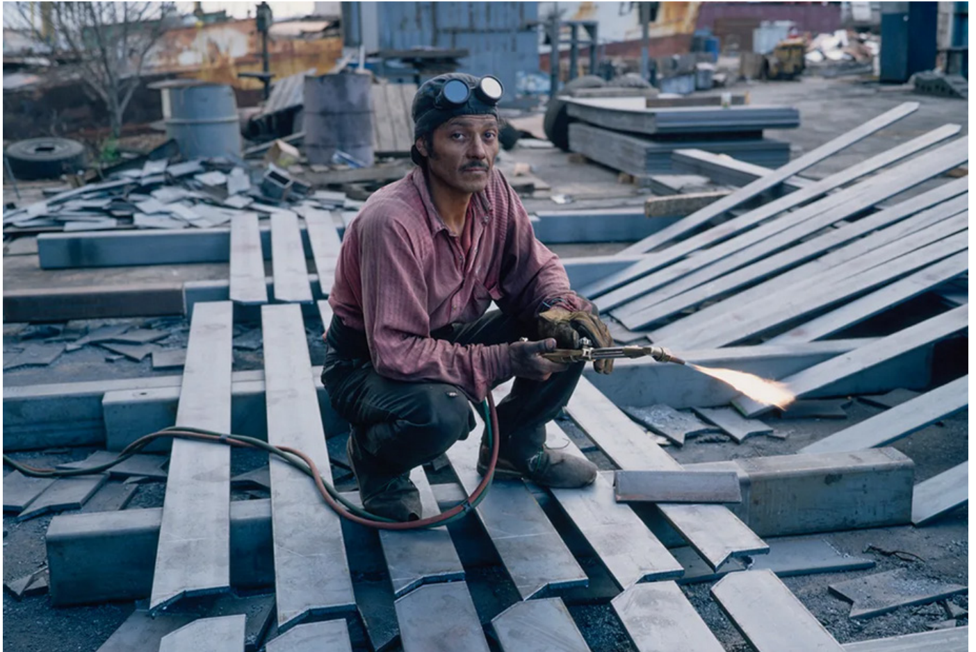
Shipyards welder cutting steel for Hyundai truck chassis, Ensenada, 1996-1997
